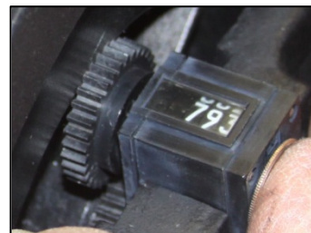
Figure 5: Pushing the Counter in; Dime used to support the Counter Shaft
