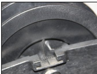
Figure 3: Spool rib aligned for install
