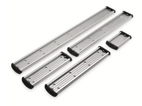
Pairs of holes are 5" on center. The holes are pass through holes for  $\frac{1}{2}$ " hardware, included hardware is  $\frac{1}{2}$ "-14 x 1.25", a 5/64" pilot hole is appropriate in most mounting surfaces. End caps are held in place by (1)  $\frac{1}{2}$ "-20 x .375" screw at the midline of the track.
